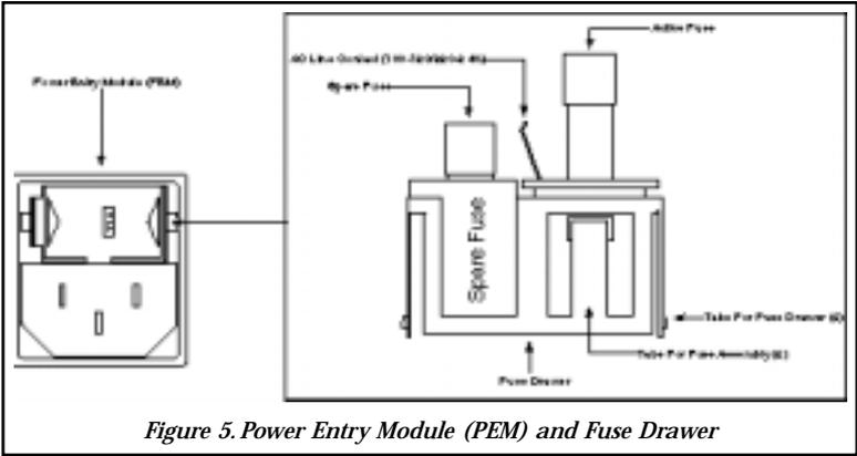
Figure 5. Power Entry Module (PEM) and Fuse Drawer
